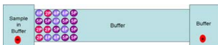
Figure 1: Sample in buffer is placed at the cathode and 20kV is applied for 10 minutes to selectively draw the anionic species into the capillary. Peptides with 2, 4, and 5 phosphorylations are represented by 2P, 4P, and 5P respectively. Their location within the capillary is meant to be indicative of their relative mobilities.
