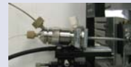
Figure 4: Agilent CE-ESI-MS Sprayer interfaced with a Micromass Q-ToF Micro. The Agilent sprayer is attached to the Micromass stage by a custom aluminum plate
